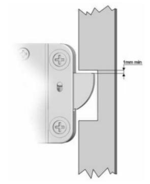
In the LOCKED position the distance between the DirectXion bolt and the boltwork part that is moving the lock bolt should be approximately 1 mm.
